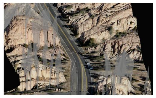
Figure 5 - MineSight oblique at Twisted Trail showing mapped discontinuity planes relative to the roadway location
